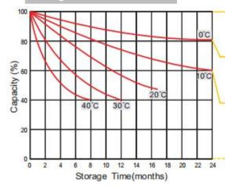
Supplementary charge required (Carry out supplement charge before use if 100% capacity is required
